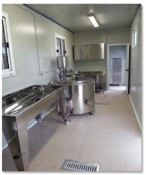
The mobile dairy is made up of: refrigerated tank for milk storage, multifunction for pasteurization and heating of milk, stainless steel processing benches, refrigeration chamber for cheese storage.
